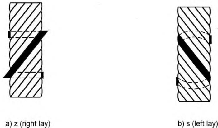
**Figure 30 — Lay direction of strands for stranded ropes**
