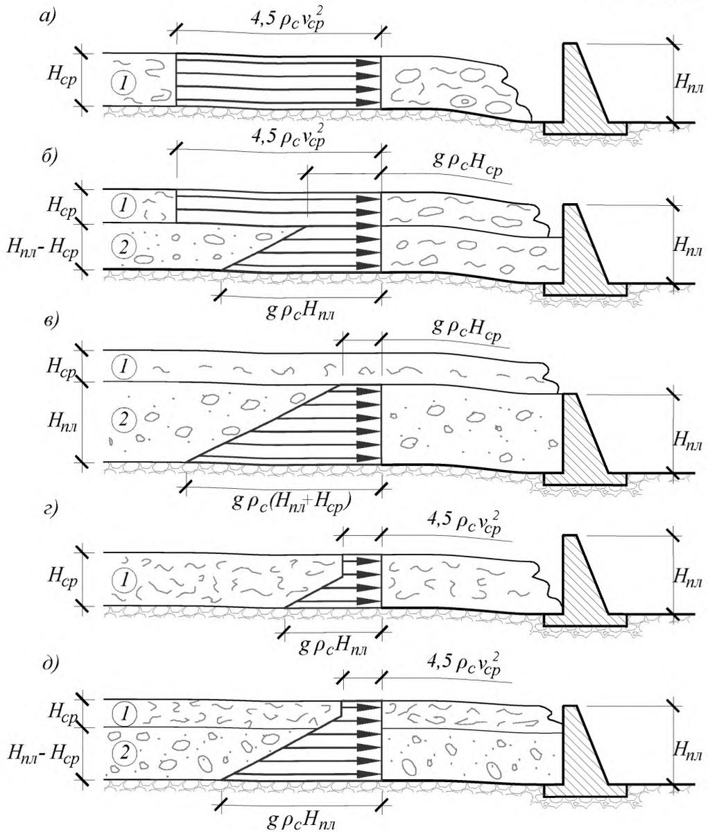
*а, б, в* – при  $4,5\rho_c v_{сп}^2 > g\rho_c H_{сп}$ ; *г, д* – при  $4,5\rho_c v_{сп}^2 < g\rho_c H_{сп}$
