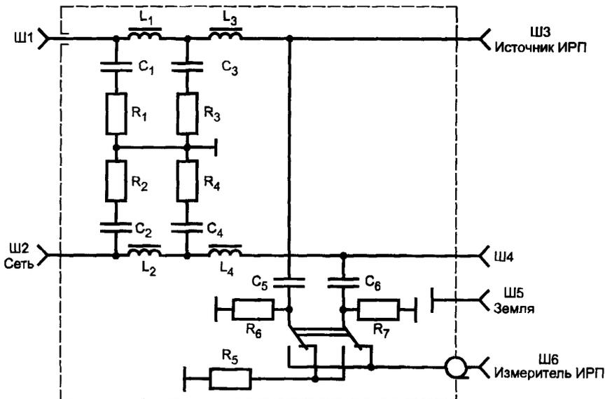
$$C_1 = C_2 = 4 \text{ мкФ}; C_3 = C_4 = 8 \text{ мкФ}; C_5 = C_6 = 0,25 \text{ мкФ};$$
