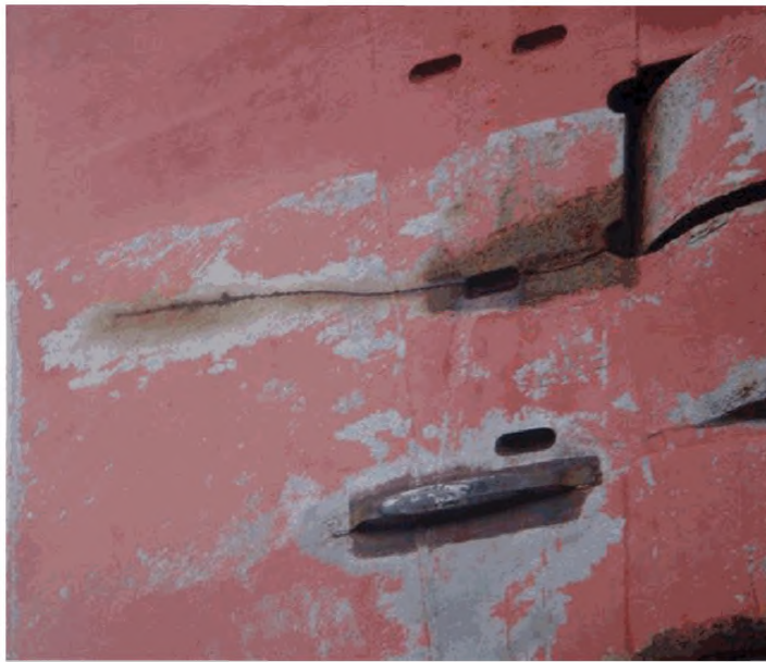
Photograph 1 Fractured rudder due to corrosion in rudder plating
