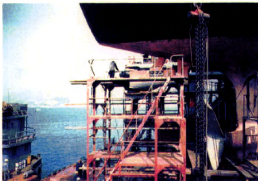
Photograph 1 Fractured rudder due to corrosion in rudder plating
