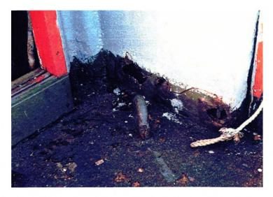
Photograph 1 Corroded accommodation house side structure
