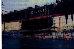
Photograph 2 Missing side shell structure (See Examples 4 and 5)
