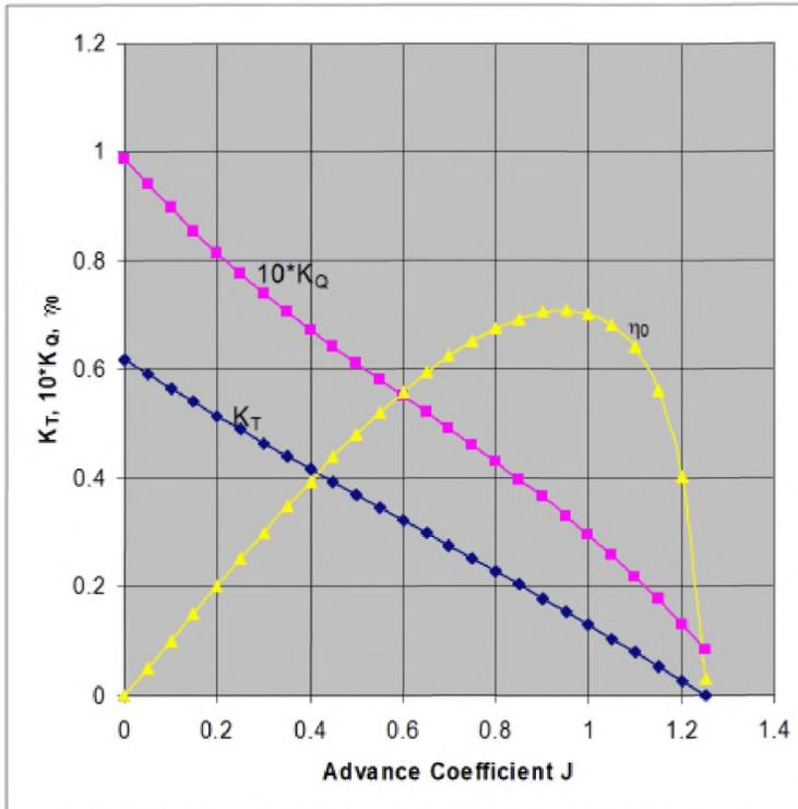
Figure 7.1: open water characteristics of ship propeller
